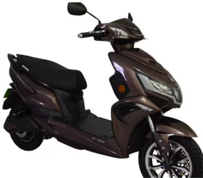
Praise Pro is powered by a 2.08 kWh detachable lithium-ion battery. ( Praise Pro )
